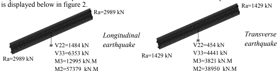
Fig. 2: Longitudinal and transverse earthquake SAP2000 load results for bridge with 30° skew angle
