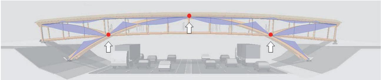
Fig. 1. Bending stress diagrams
