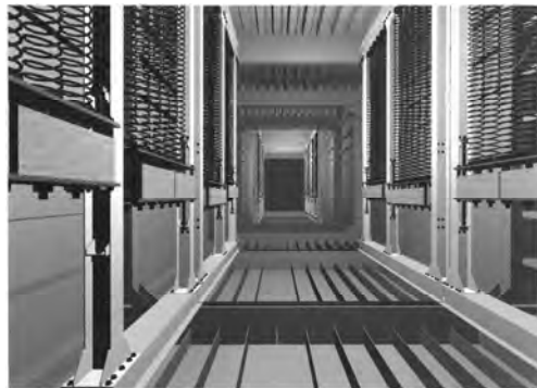
Fig. 4. View in perspective of the MSDA inside one of the box-girders.
