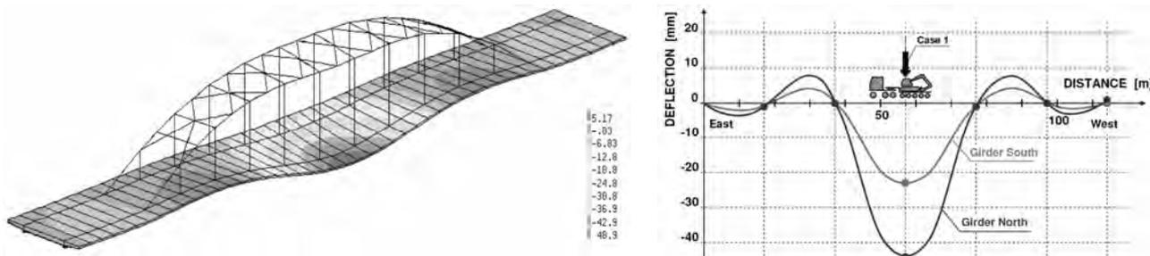
Fig. 2: Bridge analytic (left) and measured (right) deformation from vehicle in middle section
