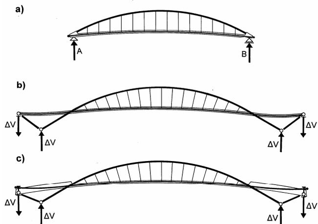
Fig. 2 Stress ribbon suspended on arch
