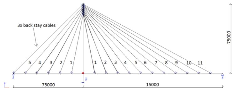
*Fig. 2: Longitudinal section of the cable stayed bridge*
