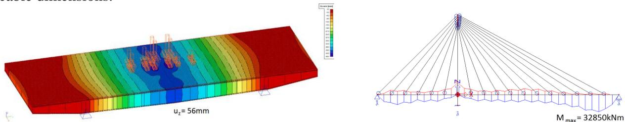
Fig. 3: FEM models (SCIA Engineer) for calculating deflections (SLS) and moments (ULS)
