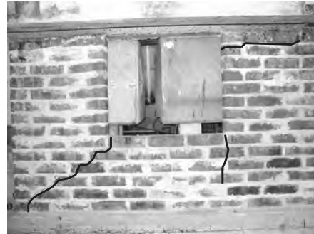
Fig. 2: Un-strengthened masonry wall failure and crack pattern
