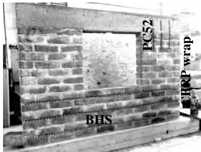
Fig. 3: Masonry wall strengthening
