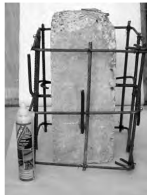
Fig. 1: RC columns strengthened by RC jacketing
