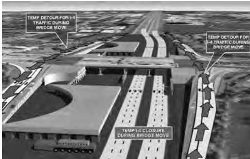
Figure 1: Bird's Eye View of Off-site Bridge Construction Scheme
