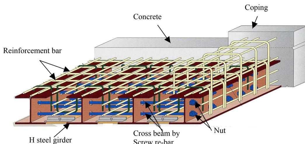
Fig. 1 General drawing of easy slab bridge structure
