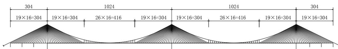
Fig. 1: Structural arrangement of the multi-span cable-stayed suspension bridge(m)
