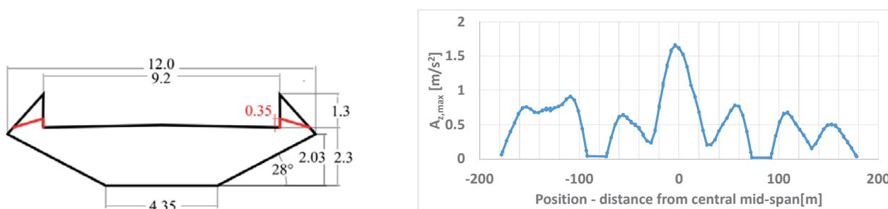
Fig. 2. On the left, Original and Tailored deck cross section (in red); on the right, example of time history analysis results.
